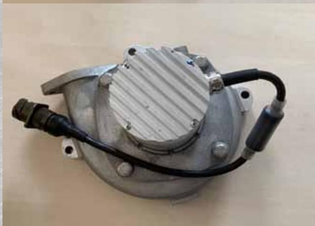
The way the blower housing is designed allows it to be fixed using different fixing options; the eyelets for 8 mm diameter screws, if unused, are all removable in order to reduce the overall dimensions to a minimum.
