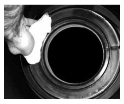
Inspect the new filter element<sup>2</sup> for damage and insert into the housing.
