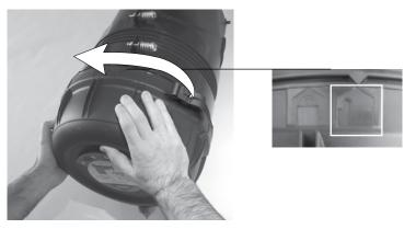
Twist the end of the filter to disengage seal. Gently remove the filter element from the housing. Inspect the
