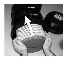
Place the OptiAir cover back on the housing.
