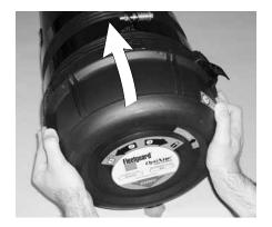
Twist the OptiAir cover to the right into the "locked" position
