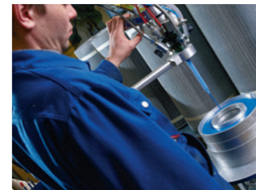
Precise moulding of end caps
