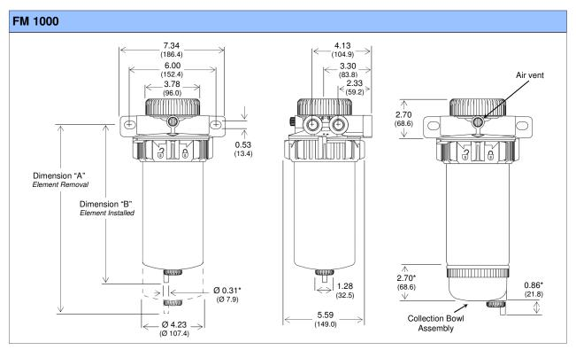
$<sup>^{\</sup>star}$  Drain Valve dimension vary with type, these are average dimensions. Applicable for FM1, FM10 and FM100
