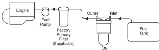
**NOTE:** Allow 3 1/2 inches vertical clearance below the unit for servicing the element and draining the contaminants.
