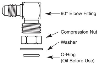
**Note:** Mount Model Before Installing Fittings. O-Ring Seal Fittings Require Care in Installation. DO NOT OVERTIGHTEN. See Instructions Below.
